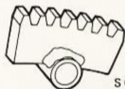
8392987 Locking segment for locking of crankshaft
