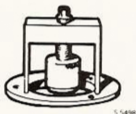
8392649 Installing and removing tool, water pump (later design)
