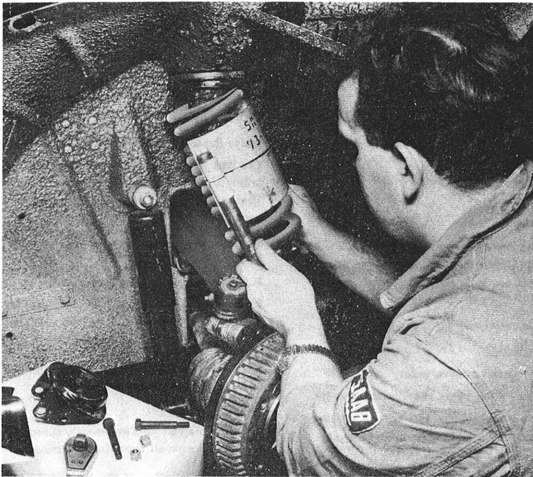
Fig. 15. Removal or installation of front spring using the tool 93-133.
