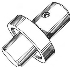
Saab 92-34 Tool for pressing rear wheel hub outer ball bearing out or in. Can also be used for pressing in seal ring around inner drive shaft in differential case if shaft is removed.
