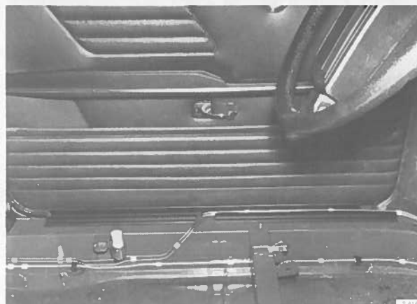
Drain holes in the sills
