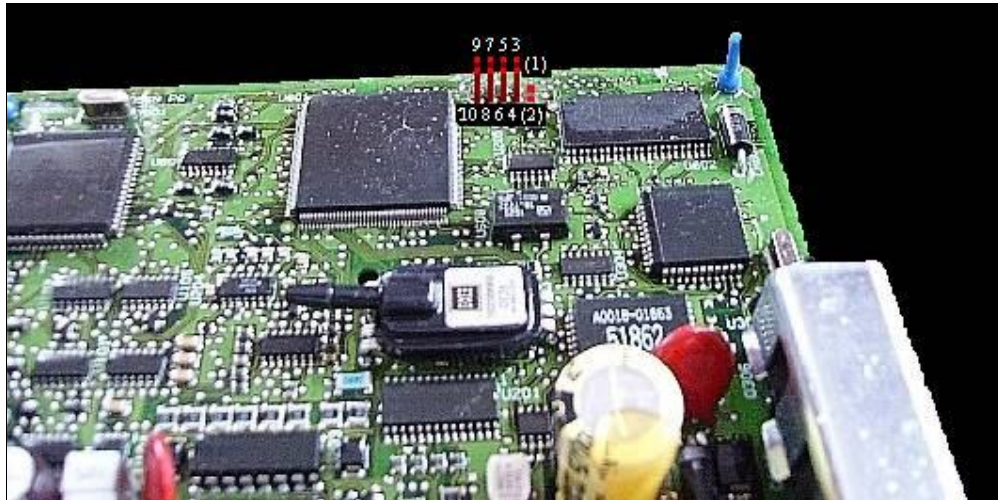
The BDM connector on the T7
